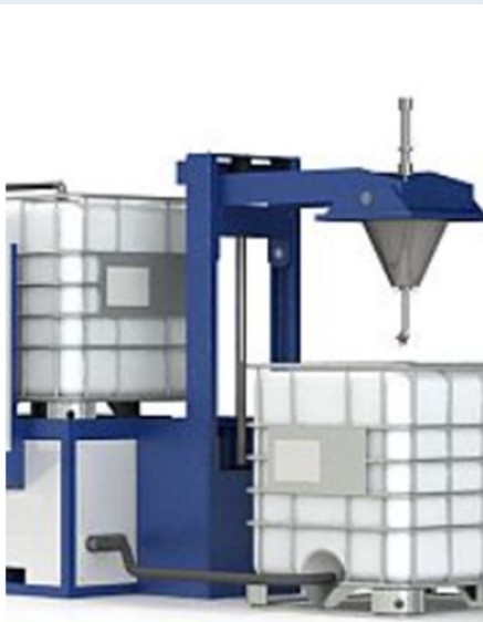
Multiple flushing of IBCs
